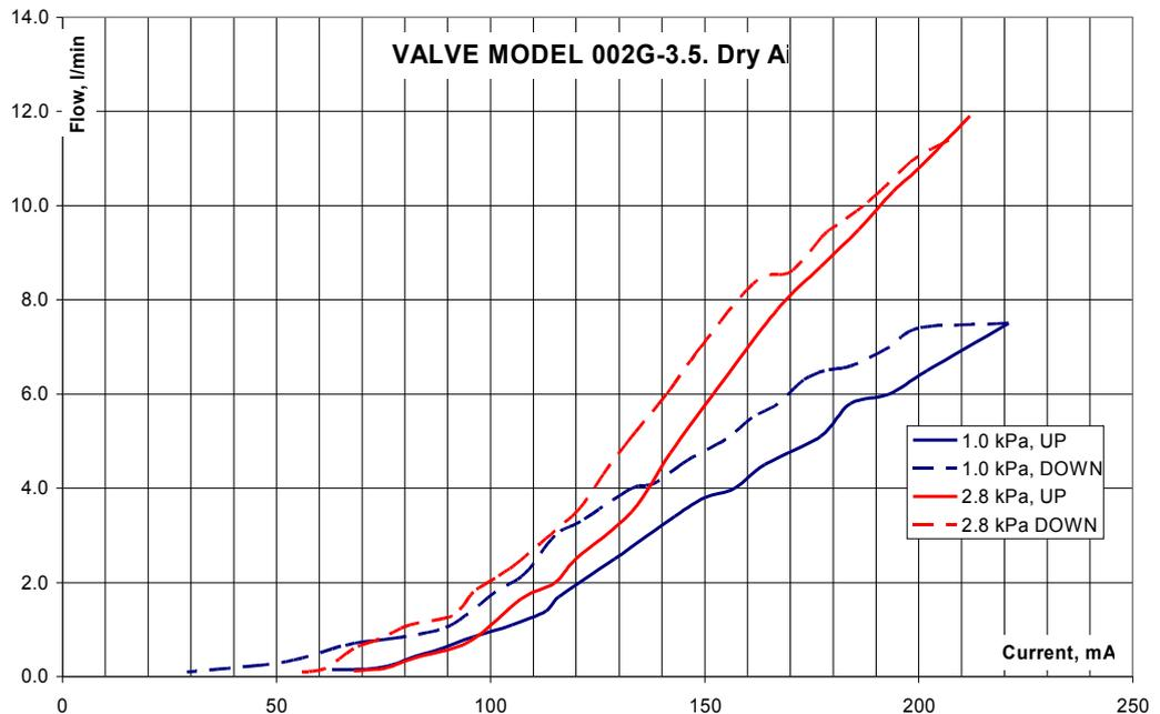
The discrepancy between the "UP" and "DOWN" curves is due to the **hysteresis** which is intrinsic to all electromagnetic devices. If necessary, this effect can be reduced by some design changes or could be dealt with electronically. Also the hysteresis effect is reduced by the limiting factor of a burner jet (injector) orifice.
